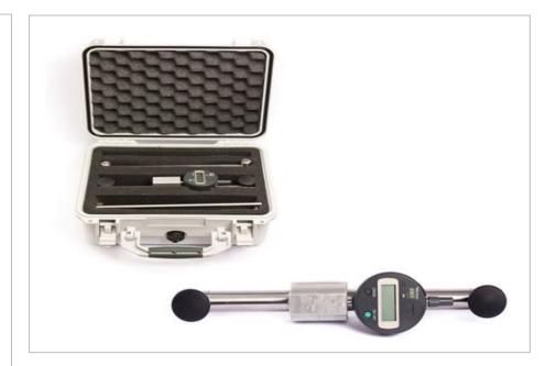
The mechanical deformometer is a measuring tool to assess changes in the distance (relative displacement) between two reading bases with order of magnitude of one thousandth of a millimetre.
