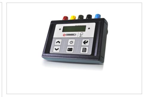
MULTIGEO (MG01) is a multi function unit designed to read on request all the main types of transducers, either electrical or vibrating wire.
