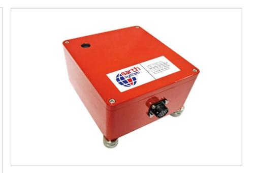
Force balance accelerometers are high sensitivity and low noise sensors designed to monitor low level low frequency seismic movements. Accelerometers are self-contained instruments and they provide high level low impedance output. Most applications do not require signal conditioning.
