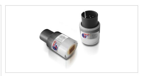
The triaxial strain cell (Doorstopper test) is made up of 3 or 4 electrical resistance sensors placed at 45 ° angle from each other. They are glued to the bottom of a borehole, previously cleared and levelled, excavated in rock or concrete.
