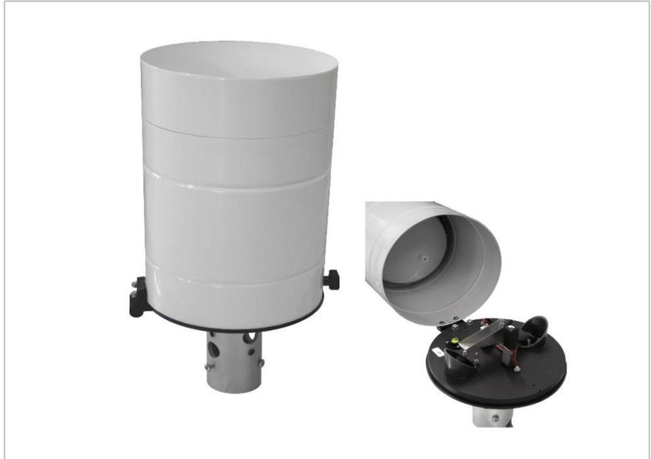
The rain gauge consists of a cylindrical body in aluminium with a collection surface of 400 cm<sup>2</sup> that houses a funnel-shaped orifice. Through a filter, it sends the rainfall collected to a tipping bucket in stainless steel with a high sensitivity knife blade support system. A reed contact detects the movements of
