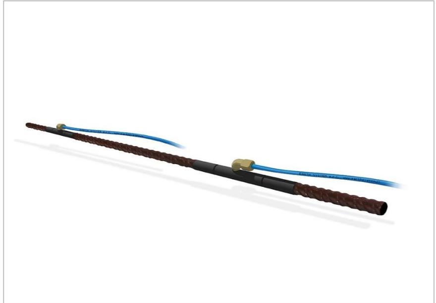
The instrumented bolt is used for measurements of strain changes in rock masses. It consists of a bar in improved bond steel with vibrating wire micro strain gauges. The strain borne by the steel bar is proportional to the axial load applied on it.
