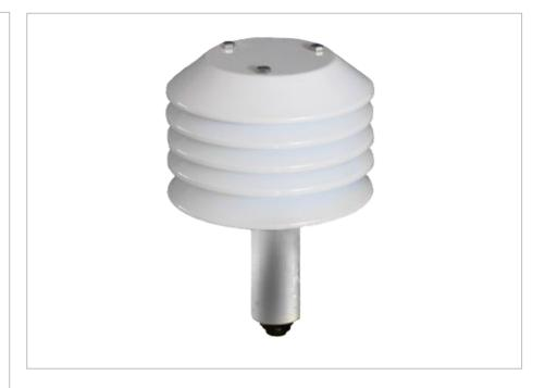
The combined Air Temperature and Humidity sensor UTA, consists of a Platinum Pt100 thermal resistance (in  $100~\Omega$  to  $0^{\circ}$ C), sensitive to the variations of temperature pursuant DIN 437601/3DIN regulation. The sensor is protected against direct sun light and UV radiations by a series of shields placed to ensure natural ventilation.
