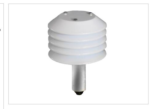
The sensor for measuring temperature consists of a Pt100 platinum resistance thermometer (from 100  $\Omega$  at 0°C), sensitive to temperature variations according to DIN 437601/3DIN standards.
